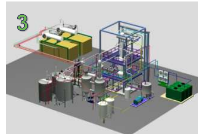
Alphakat Plan with connection to diesel tanks
